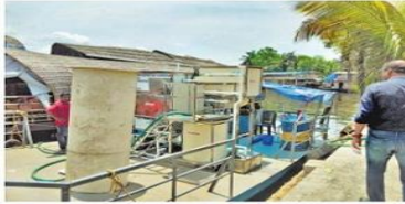
The mobile septage processing unit introduced by the Kerala State Pollution Control Board | Express
