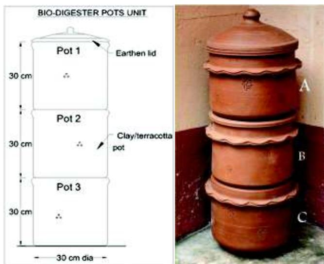
Figure 3: Specifications of Khamba or 3 vessel composting
