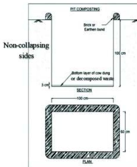
Figure 1: Specifications of Pit Composting
